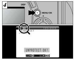
When you press the "MENU/OK" button, the image is protected and the "" icon appears on the screen. To remove the protection, press the "MENU/OK" button again.
